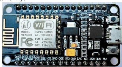
Fig. 5. Appearance of the Wi-Fi module- ESP8266EX
